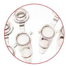
**SnapStrip** single interwell linkage makes strips easy to split into smaller sections.
